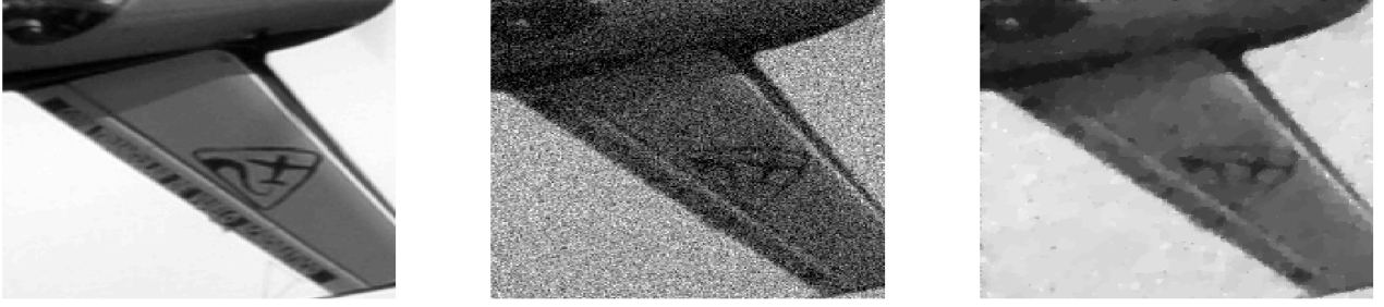
Figure 17: Poisson-Gaussian denoising: Original image (left), noisy image corrupted by Poisson noise and Gaussian noise with mean zero and variance 0.001 (center) and denoised image (right). Optimal parameters \lambda_1^* = 1847.75 and \lambda_2^* = 73.45 .
