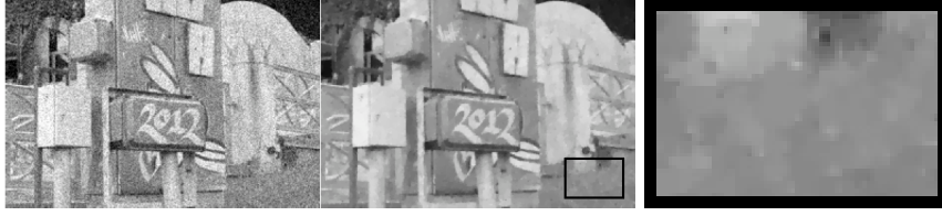
Figure 3: TV image denoising and the staircasing effect: (l.) noisy image, (m.) denoised image, (r.) detail of the bottom right hand corner of the denoised image to visualise the staircasing effect (the creation of blocky-like patterns due to the first-order regulariser).
