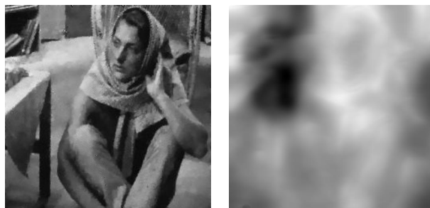
FIGURE 4.4. First row: Denoised image (left) and image form of \lambda (right).
